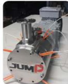
JEB1.1s with casing and heating resistors
